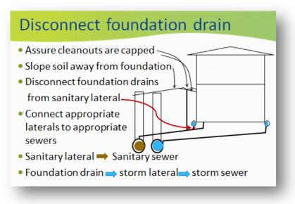
Now you must disconnect foundation drain and any other clean water sources from your existing sanitary lateral, and most likely run a new storm lateral to the lateral stub at property line.
